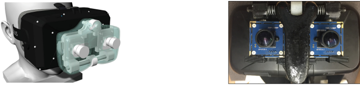
Fig. 1. (left) CAD model showing the camera attachment. (right) 3D printed attachment on the Oculus Rift.
