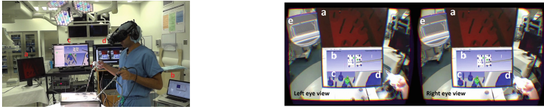
Fig. 3. (left) User with the MRNLS performing the trial (right) view provided to the user through the HMD. Virtual monitors show the laparoscopy view (panel a - red hue) and the navigation system display (panel b, c, d). The surrounding environment (label e) can also be seen through the HMD.
